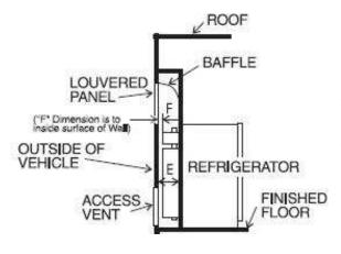
We finished the conversion of the fridge compartment to match the Dometic spec by using a piece of sheet panel to create the rounded roof (baffle on diagram) for the upper cooling vent. The triple fans were then place to cover the upper vent. The spec for "F" is 1 inch between the fins and the wall. Originally this was
